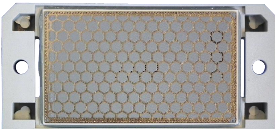
Figure 2: Pattern after screen printing
